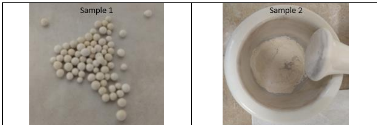
Figure 3. (left) Sample 1 – Pelletized Zeolite 13X (right) Sample 2 – Crushed Zeolite 13X
