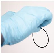
6. Place the O-ring back into the groove with the greased index finger, gently pressing it back into position.
