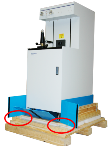
Support studs for ramp
