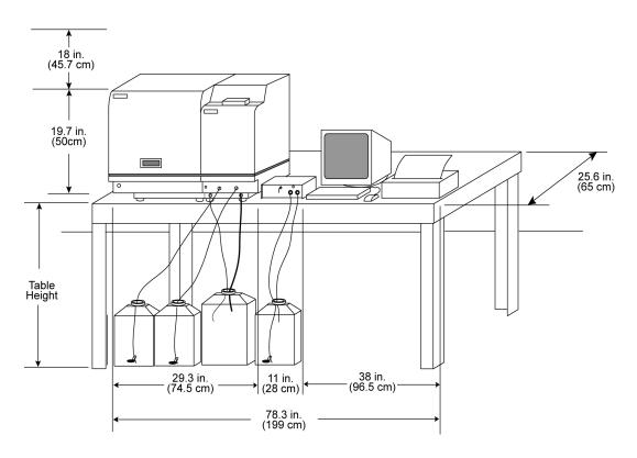
The height of the Saturn DigiSizer 5205 and LSHU is 19.7 in. (50 cm). An additional, 18 inches (45.7 cm) is required for clearance when the front door is opened (raised). Inspect the area above the combined heights of the analyzer and table to ensure the absence of lab cabinets, air ducts, pipe, light fixtures, etc.
