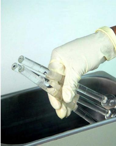
5. Use rubber gloves to ensure no oils or residue are transferred to the clean tubes and filler rods, then remove the sample tubes and filler rods from the unit.
