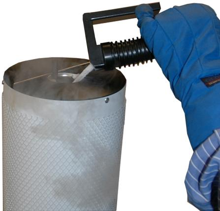
1. Fill the Dewar with the analysis bath liquid (such as liquid nitrogen) to no higher than 2 1/4 in. (5.7 cm) from the top. Filling the Dewar higher than this will cause an error in the free space measurement.
