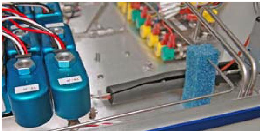
6. Place the heated manifold cover over the analysis manifold and secure with the two screws removed in step 2.
