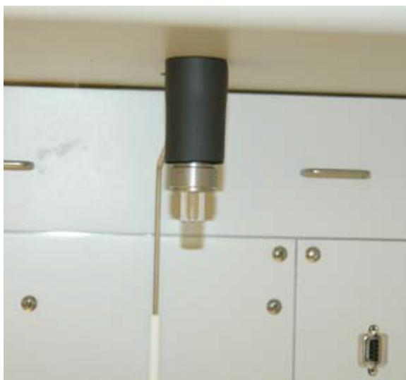
1. Remove the sample port connector nut.
